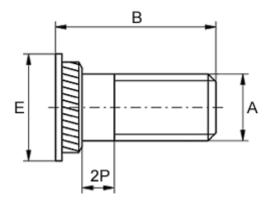
For plate thickness, min = 1.5 Head diameter E = 8 Hole diameter +0.1 = 6.4 Length B = 16 Male thread A = M5x0,8 Min distance to edge = 3.3
